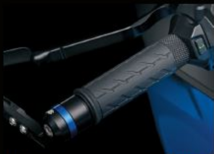
Grip Heater 57100-48821-000 With three different heat settings.
